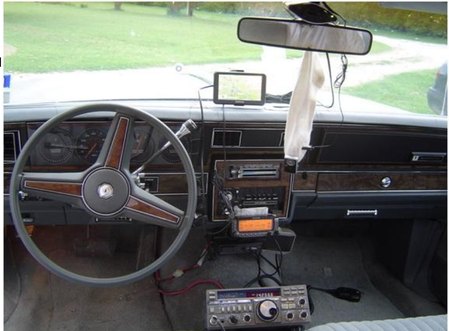
INSIDE WBØTEV/M: DashCam atop rearview mirror, Sansa Clip & DashCam mic on sock dangle above the FT-757
